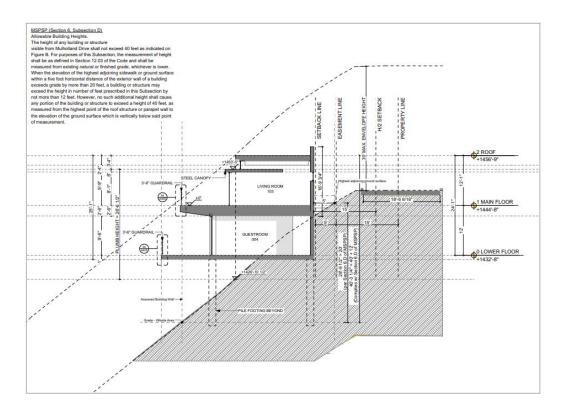
Please note that on the Northern end, we have a 1 story garage and a big deck area at a lower elevation. The project continues to step down along the N/S axis and the steepest portion of the lot (Southern end) is left undeveloped and with a big balcony to set back the roof structure. The entire building is broken up in many different levels to achieve this while achieving on of the most important MDRB guidelines: blending the project with the surrounding and the Santa Monica Mountains.
